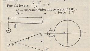
Ex.—If the distance from the fulcrum of a lever to the weight is 3" and the weight to be raised is 200 lbs., what length should the long arm of lever be with a force of 30 lbs.? Also what force would be required if the long arm were 24" long? (Back face) Set 3" on B to 200 lbs. on A. and under 30 lbs. on A read 20" length of lever on B, and over 24" length of lever on B read 25 lbs. on A.
